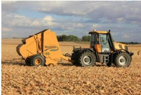
One version of Vermeer’s 605 corn stover special lays bales out across the row. The goal of field testing is to identify the technology that speeds up and improves the efficiency of biomass collection.
